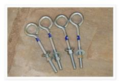
Prepare the eye bolts by adding the large washer, then the nut. These help give the concrete something to hold onto, so that the eye bolt won't pull out of the concrete over time.
